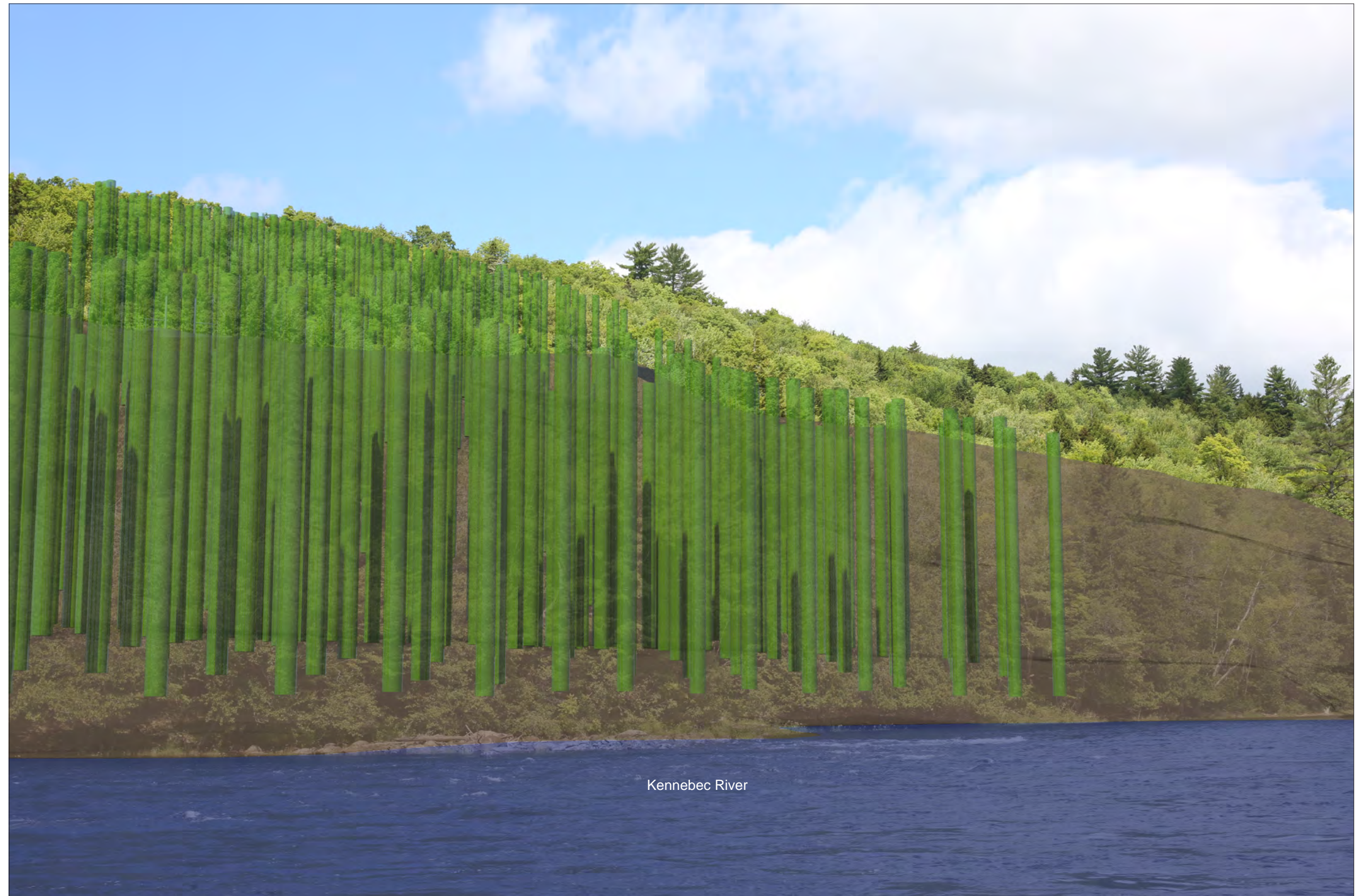
COMPUTER MODEL A-3: This image shows the computer model (terrain and 75' tree cylinders) overlaid and registered with the Existing Conditions photo. The preserved vegetation on the hillside will completely screen the West Forks Termination Station from the Kennebec River.
